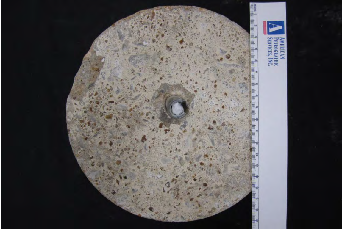
SAMPLE ID: B7 DESCRIPTION: Top surface of the sample as received. Note the mortar eroded surface.
