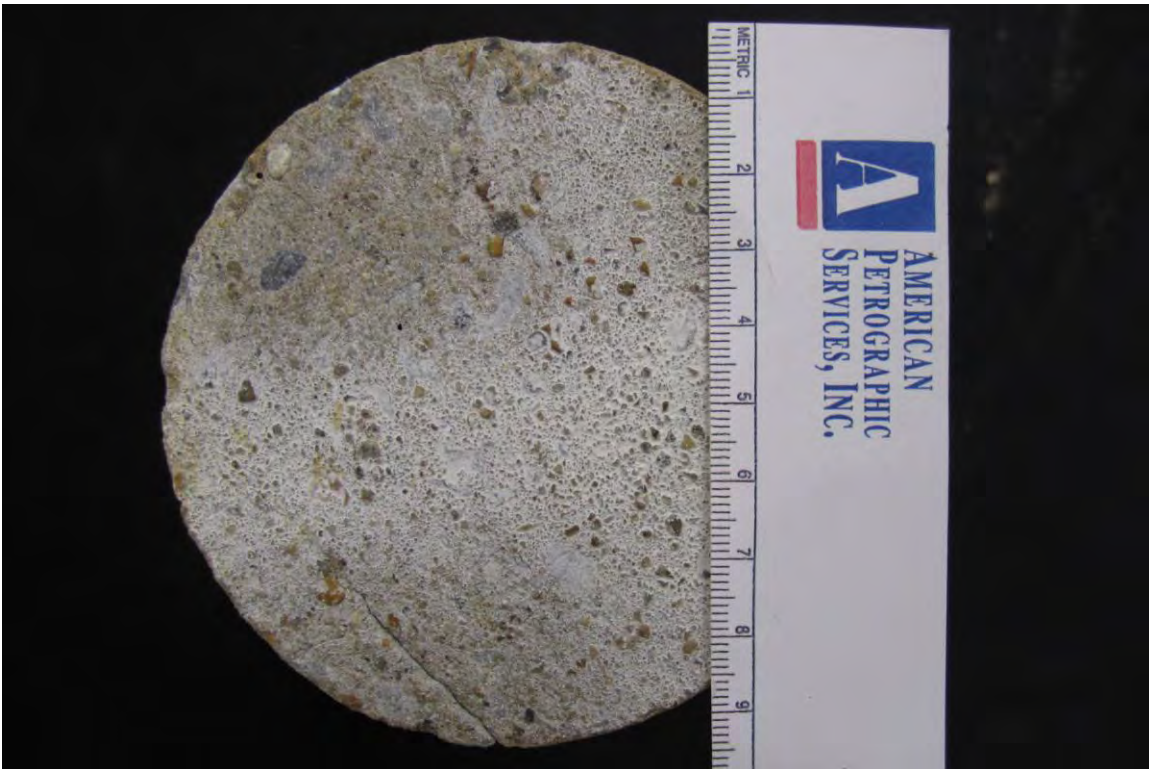
SAMPLE ID: P14 DESCRIPTION: Top surface of the sample as received. Note the mortar eroded surface.
