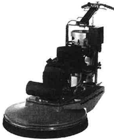
Figure 36 High Speed Burnisher with dust control
