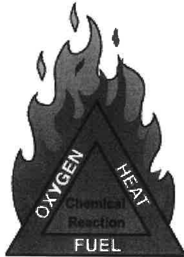
Figure 13 Oxygen Heat and Fuel Triangle
