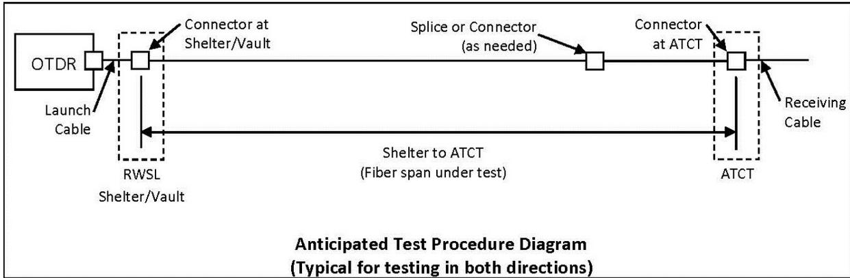
Provide printed and electronic copies of OTDR traces (including source program if necessary to read), and documentation of all testing in report form to the RPR for review. Include wavelengths, fiber type, fiber identification, measurement direction, test equipment model and serial numbers, date, reference setup and operators.
