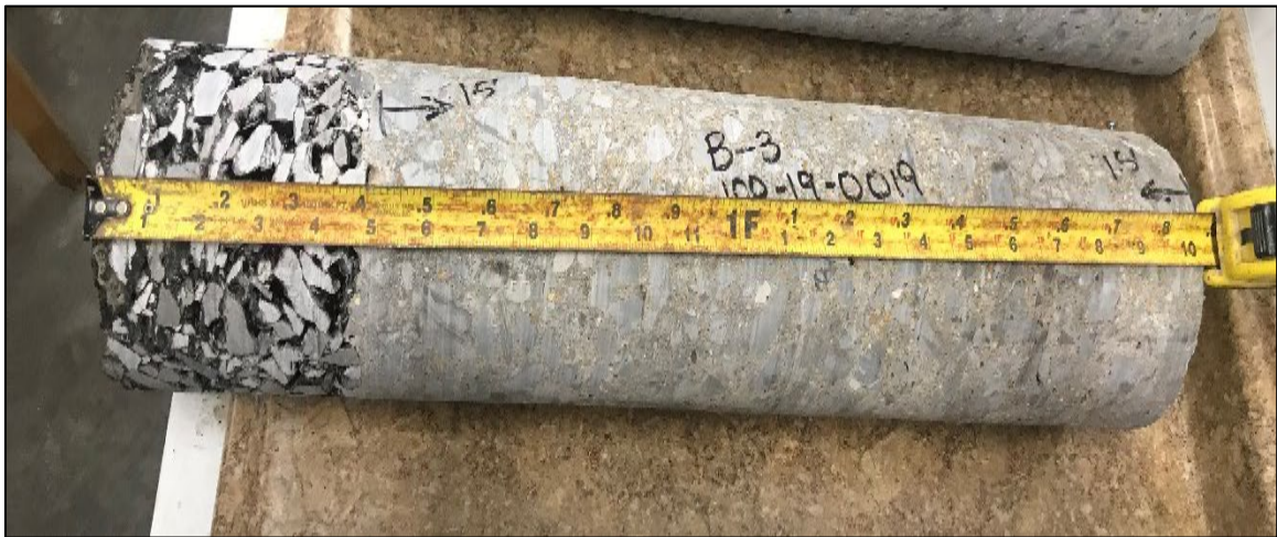
Photo 11: Concrete Core Location B-3
