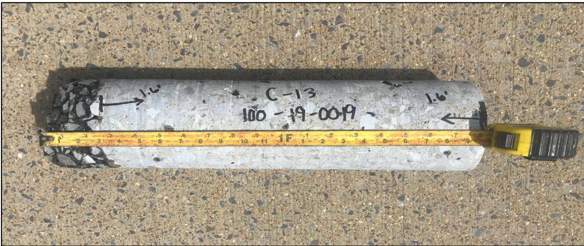
Photo 8: Concrete Core Location C-13
