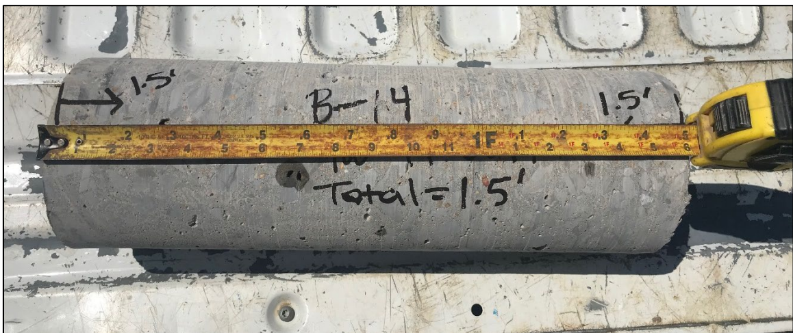
Photo 21: Concrete Core Location B-14
